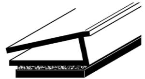
**ADD-ONS AVAILABLE** - Magnetglaze Heavy Duty Sash Kits - make your Magnetglaze Pro frames into 2 or more panels with a sash kit that uses a specially designed jointing strip to maintain the thermal seal between panels. Please note that the Sash kits are designed for 4mm plastic sheet only.
